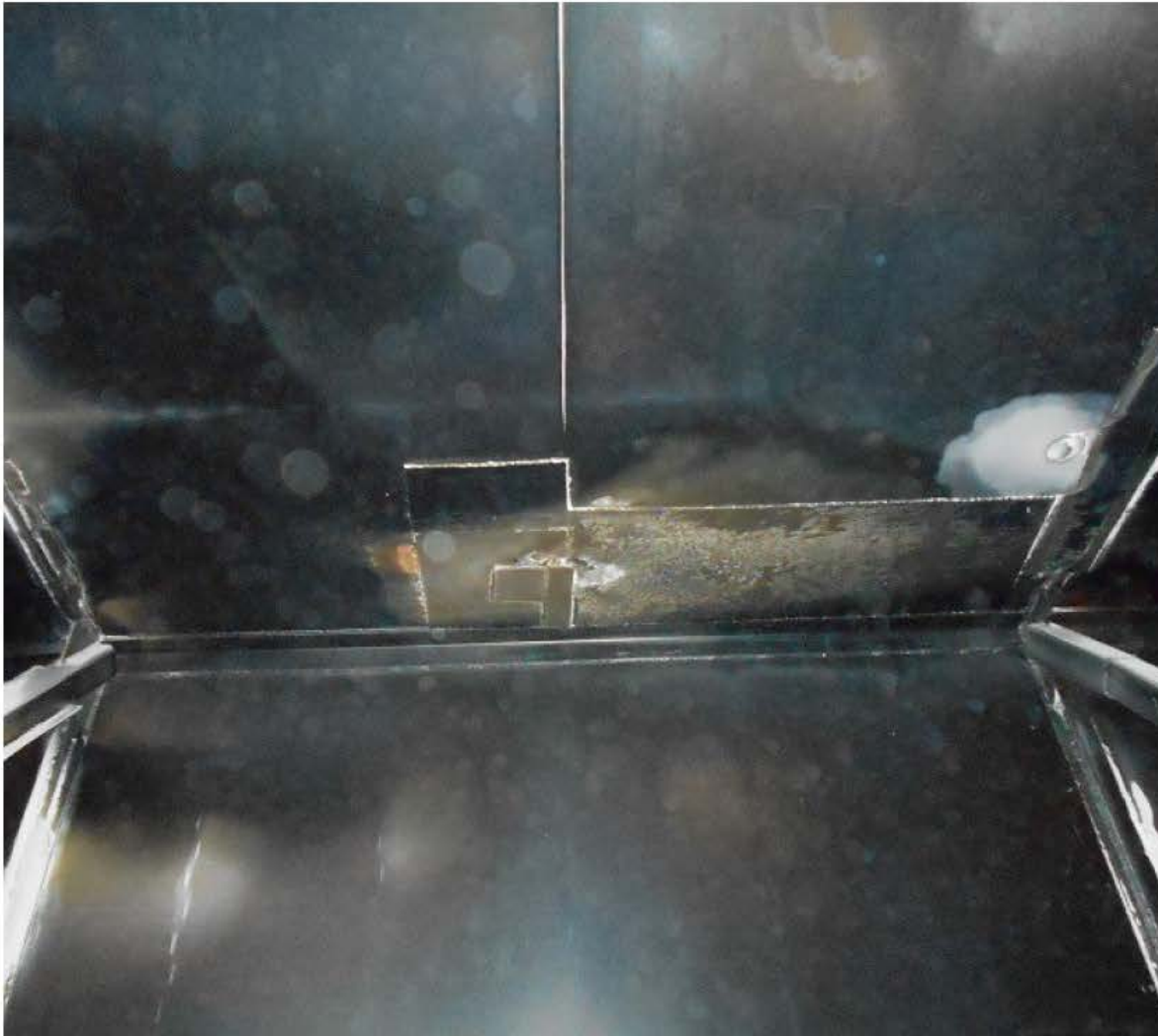
Duct roof erosion downstream of mixers, near unit centerline (flow is left to right) (zoomed view at right; repair patches evident)
